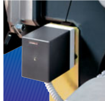
Example of the servomotor for air/oil setting
